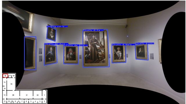
Figure 1. Example of the final result of our image processing pipeline using standard computer vision techniques. The image is undistorted, the paintings have been detected and recognized. The room has also been localized.
